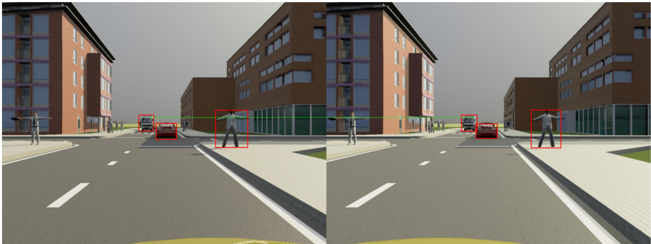
Figure 35: Object Correspondence via matched keypoint in left and right images
